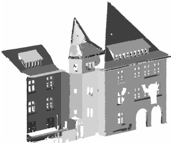
Figure 18: Adjacent façades segmented into principal planar surfaces and features
