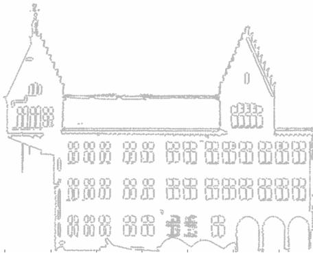
Figure 17: Contour points extracted from the façade depicted in Figure 16
