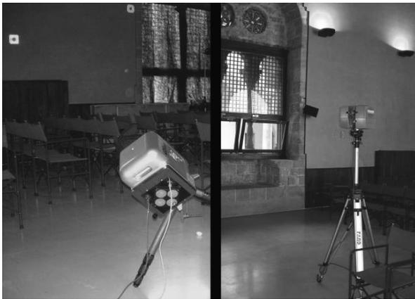
Figure 4. Laser scanning survey. *Left*: Mensi GS 200 and reflecting targets on the wall. *Right*: Faro LS880
