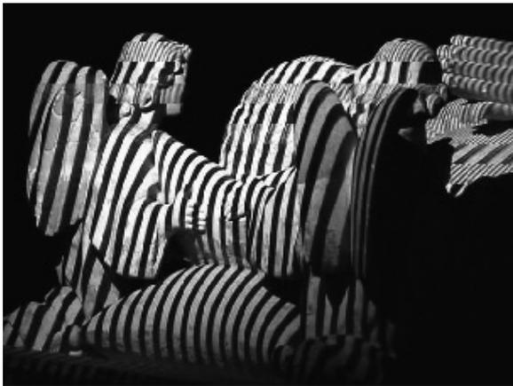
Figure 3: Digitization of the recumbent shape using a structured light device.
