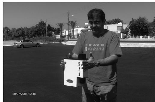
Figure 3: SCV HR-1024 Field Spectroradiometer
