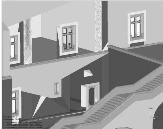
Figure 8: Built 3D model, views over the interior. The windows were redrawn based on scanned 3D data (window fragments).
